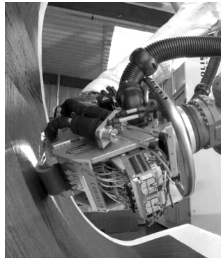
Automated Fiber Placement
