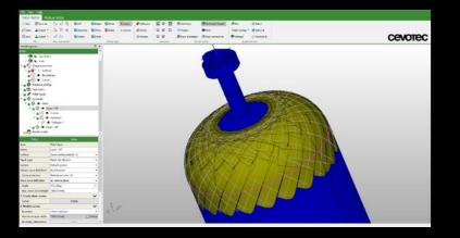
PATCH ARTIST is the patch laminate design module. Its user interface is designed to define patch zones easily on imported CAD surfaces, as well as layer orientations, tape thickness, tape width, patch overlaps, patch length and patch side angles.
