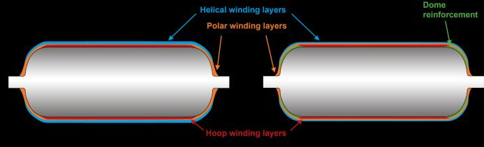
Dome reinforcements replace certain helical layers in a winding laminate
