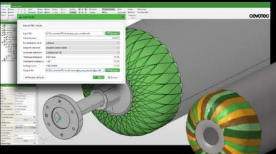
ARTIST STUDIO support for FE-modeling automatically generates a detailed FE-model of the patch laminate based on the data defined in PATCH ARTIST regarding geometry, position and orientation of the patches.
