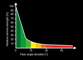
Example: 15° deviation between fiber orientation and load results in approx. 80% reduced fiber strength.
