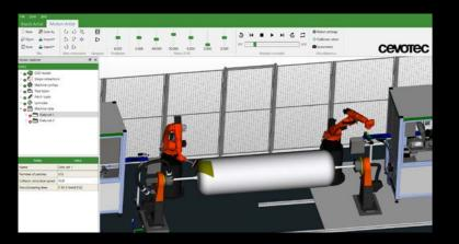
MOTION ARTIST enables you to program SAMBA robots offline in a completely automated fashion. This feature significantly reduces production preparation time while enhancing safety on your shop floor through built-in collision detection and visual process simulation.
