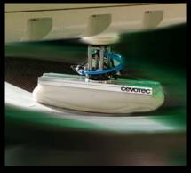
Form-flexible patch grippers support the automated and precise fiber lay-up for monolithic and sandwich components.
