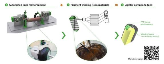
This approach reduces net fiber consumption by approx. 15 % or more, depending on the vessel characteristics, which translates into considerable weight and material cost savings while maintaining equivalent mechanical properties. Due to the material reduction, the reinforced tanks also feature more storage volume in the same built space and have an improved CO<sub>2</sub> footprint.
