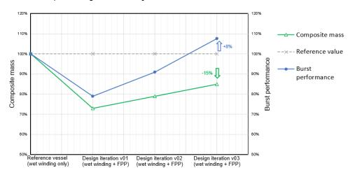
The storage efficiency is a key indicator for a pressure tank, setting the mass of the compressed  $H_2$  in relation to the total mass of the storage system. For v03, **storage efficiency is 6.1 %, which represents an increase of 17 %** compared to the 5.2 % storage efficiency of the reference vessel.
